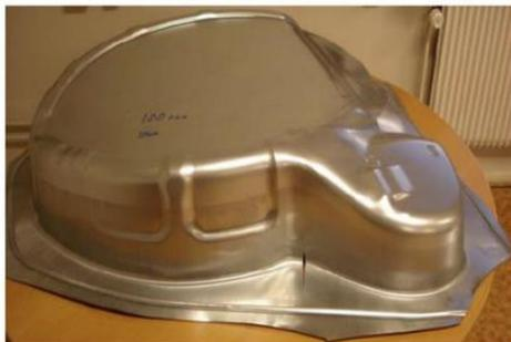
Volvo Cars component with failure after forming due to non-linear strain path
