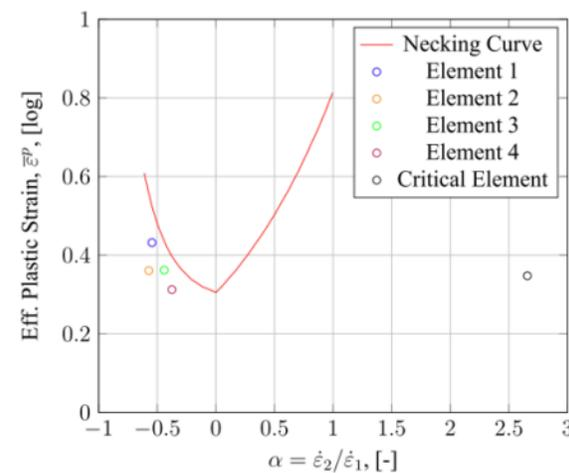
The critical element was located where fracture occurred in the component, showing a clearly non-linear strain path with a 90° turn
