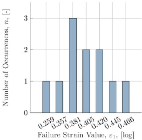
Failure strain for the surface layer in the FE model
