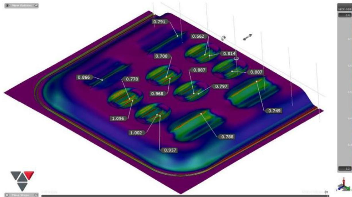
A necking index was defined that updates the failure strain based on stretching-to-bending ratio and indicates how close the element under evaluation is to necking. The necking index is calculated using the maximum principal strains of the upper and lower layers of the element of interest. Here, an index equaling to or more than 1 means the necking limit has been reached
