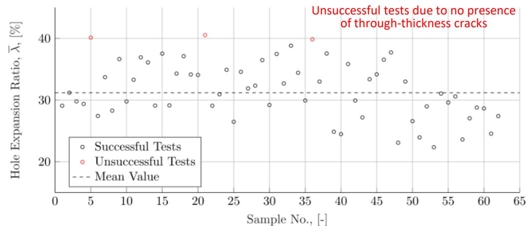
HET of the 62 tests conducted
