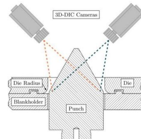
New experimental setup with draw beads and DIC system
