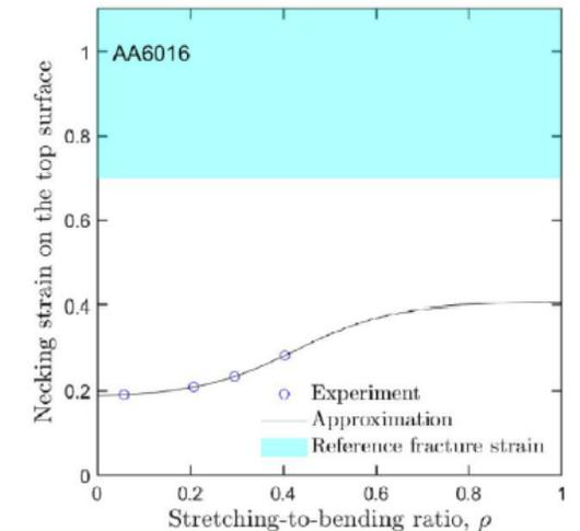
Forming limit of the tested materials under combined stretch-bending loads
