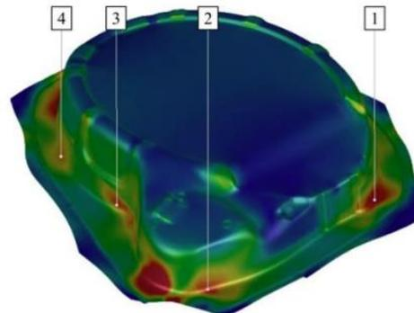
FE model with 4 arbitrary control elements in areas with high plastic strains
