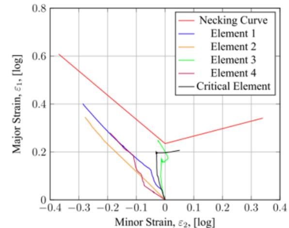
Strain paths of the 4 control and 1 critical elements
