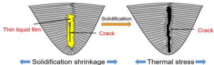
The solidification crack of the 6XXX series Al alloy
