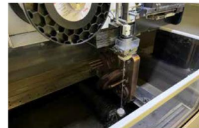
Cut-off and removal of support structures
